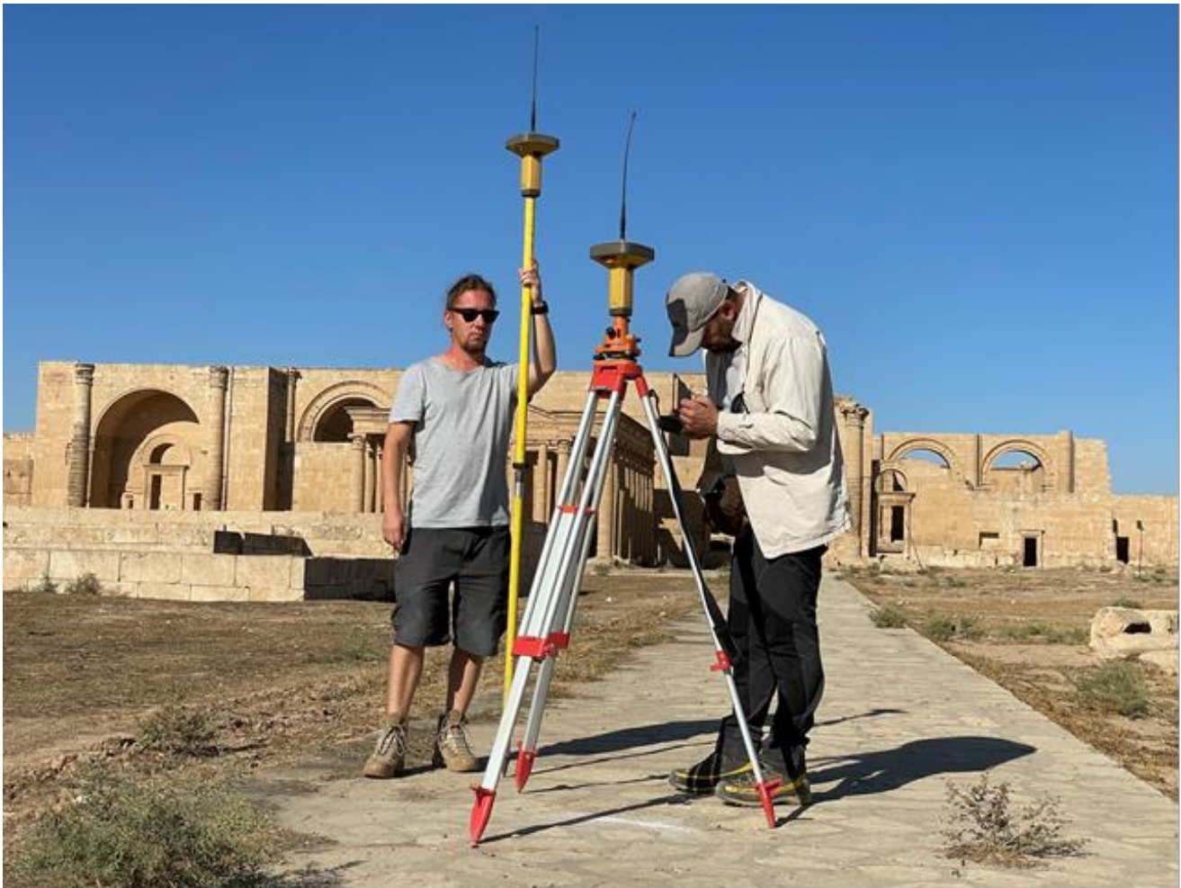
Fig. 45: Setting and measurement session of the GNSS base station and rover system.
